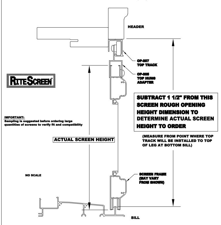
NOTE: THIS SIZING METHOD SHOULD WORK IN CASES WHERE TOP TRACK NUMBER OP-007 AND TOP HUNG ADAPTER NUMBER OP-005 ARE USED, WHILE ACTUAL SCREEN FRAME USED MAY VARY FROM THAT SHOWN. HOWEVER, IF YOUR DOOR OPENING CONDITIONS VARY FROM THOSE SHOWN, THIS METHOD MAY NOT PROVIDE ACCURATE SCREEN HEIGHT. PLEASE CONTACT RITESCREEN FOR ASSISTANCE WITH OTHER TYPES OF CONDITIONS.
