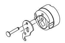
TURN THE CAM OVER AND PUSH THE CAM PIVOT PIN THRU THE CAM AND INTO THE CAM DISC AS SHOWN.
