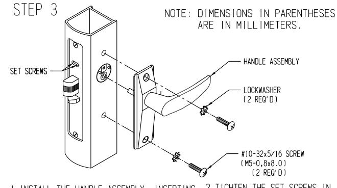
1.INSTALL THE HANDLE ASSEMBLY, INSERTING THE SQUARE SPINDLE INTO THE HUB OF THE CAM DISC. SECURE THE HANDLE ASSEMBLY WITH (2) #10 (M5) SCREWS AND LOCKWASHERS.
