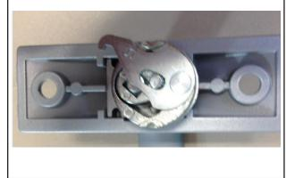
Step 2: Slip the cam off the handle, flip it over, and you see there is An E ring holding that cam on (the top of the post the e ring holds is the large circle shown at 3 o'clock in the below pic).
